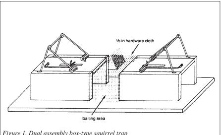
Figure 1. Dual assembly box-type squirrel trap
