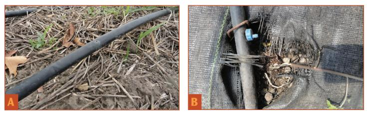
Figure 5. High-pressure drip system emitters can be (A) preinstalled at the factory or (B) installed during assembly.
