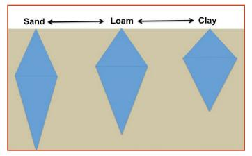
*Figure 3.* Distribution of water in various soil types. High concentrations of clay lead to wider distribution, and greater amounts of sand lead to narrow water distribution.
