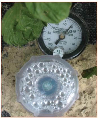
*Figure 13.* A tensiometer can be used to monitor soil moisture. feet). In this case, the tape uses 8 gpm to run the irrigation system:
