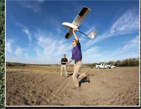
The rigid wing and streamlined shape (airfoil) lift the aircraft as it accelerates. A single propeller driven by an internal combustion engine or electric motor produces forward thrust and enough airspeed to keep the payload aloft.
