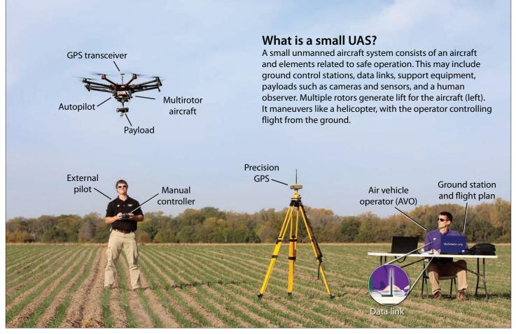
Small unmanned aircraft systems (UAS), also known as drones, are fixed-wing or rotary-wing vehicles that do not carry humans on board. The term sUAS applies to any unmanned aircraft weighing less than 55 pounds. The smallest vehicles weigh less than a pound and fit into the palm of your hand. Small, electric-powered versions can fly for 15 to 25 minutes. Larger, gas-powered models fly for up to 24 hours.
