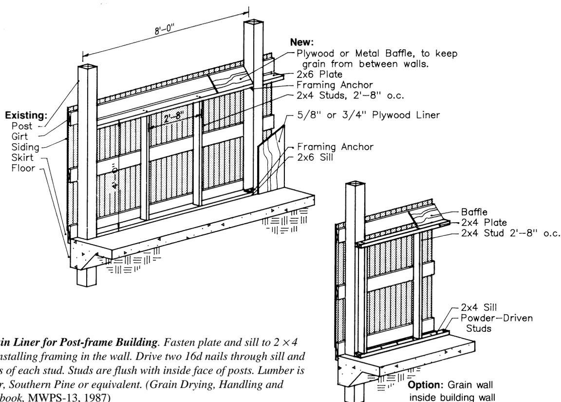
**Figure 1. Grain Liner for Post-frame Building.** Fasten plate and sill to 2 × 4 studs before installing framing in the wall. Drive two 16d nails through sill and plate into ends of each stud. Studs are flush with inside face of posts. Lumber is No. 2 or better, Southern Pine or equivalent. (Grain Drying, Handling and Storage Handbook, MWPS-13, 1987)
