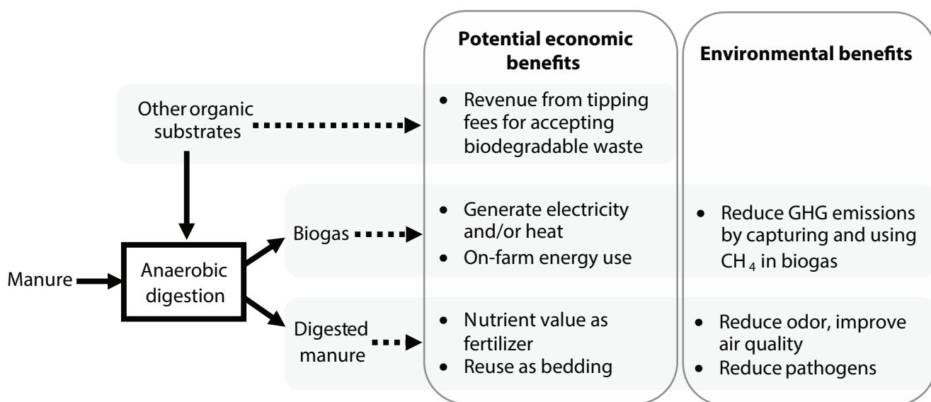
**Figure 1.** The environmental and potential economic benefits of anaerobic digestion.
