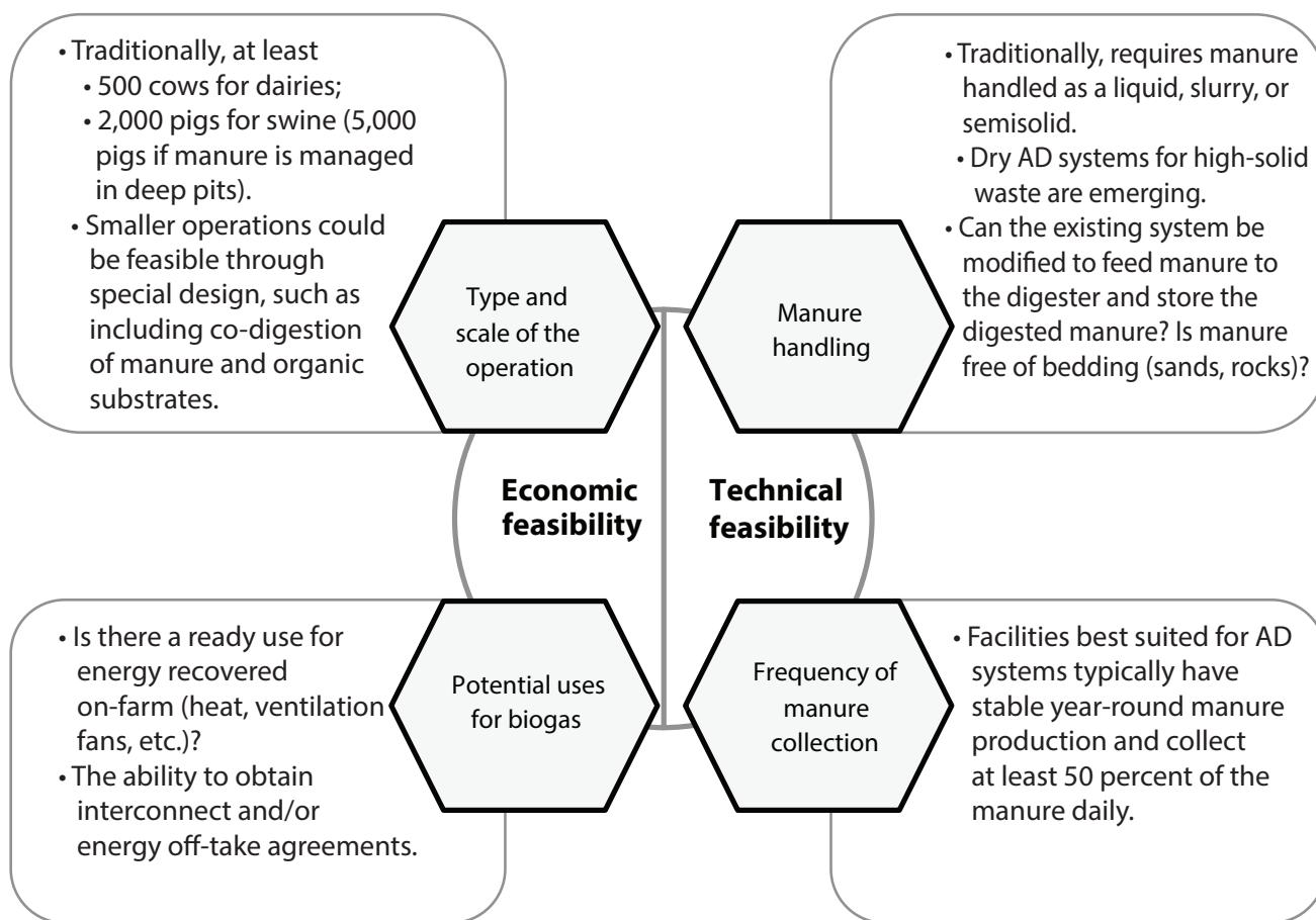
**Figure 2.** Assessing feasibility of installing an AD system for livestock operations (Adapted from AgSTAR, 2011).
