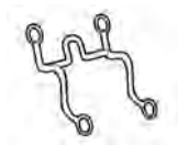
Illegal curb – port higher than 3½".
