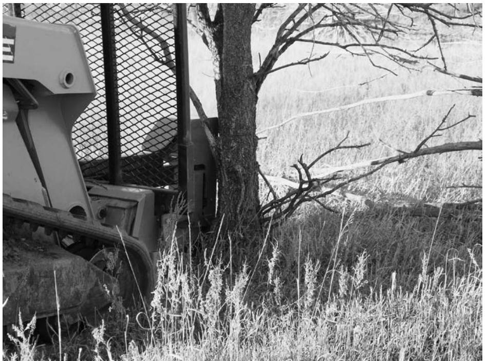
Using a hydraulic saw to cut down a tree in a pasture. Trees should be cut close to the soil surface.
