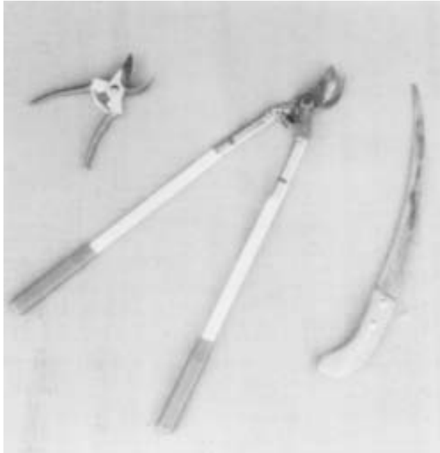
Figure 1. Necessary pruning equipment (A) Scissors type hand shears, (B) Loppers and (C) Fine Tooth Saw.
