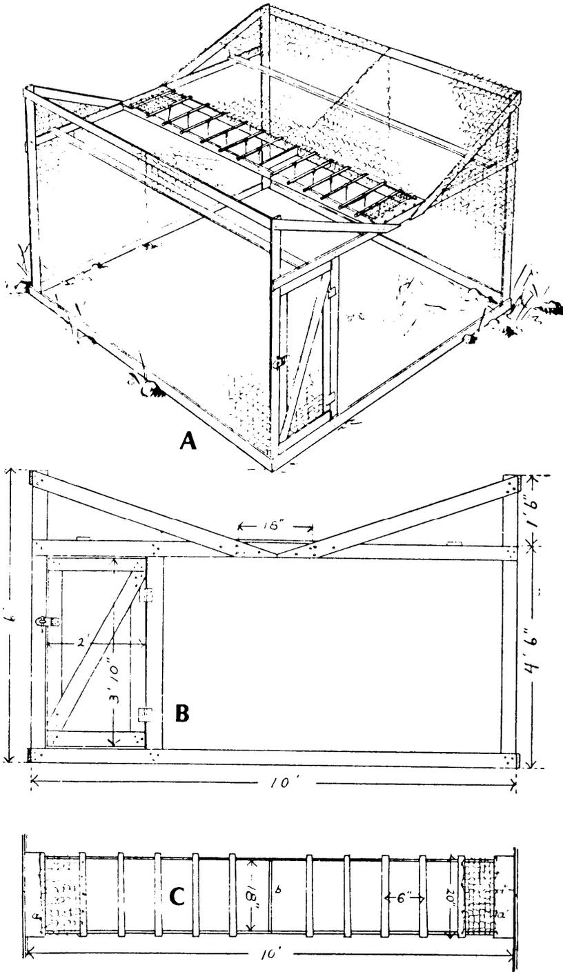
Australian crow trap: (A) completed trap, (B) end view, and (C) plan of "ladder" opening.
